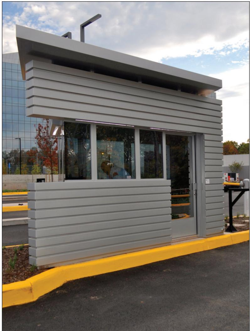
roof is finished with a three-part, Energy Star-compliant membrane boasting a solar reflective index of 95-plus. The booth's stainless steel floor sports hard-wearing commercial rubber tile. The doors are top-hung sliding, with stainless steel frame, utilizing eight 2 1/4" diameter rugged steel ball bearing rollers. A stainless steel lower guide, and welded stainless steel pull handles complete the door system.
