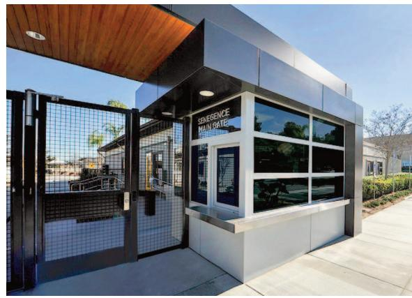
with # 4 finish, energy star rated HVAC, convenience outlets and data & communication J-Boxes, galvanized steel plate floor covered with B.I.G.'s exclusive polyvinyl chloride interlocking tiles and 4" tall base cove, and to finish it off, a high solids polyurethane paint finish over a two-part polyurethane primer. The unit also has architectural galvanized steel panels that create horizontal & vertical reveals.
