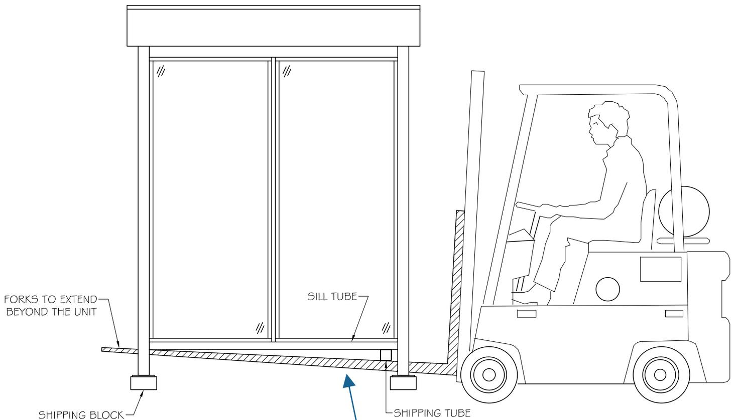
Forks angled to correct the height difference at the shipping and sill tubes
